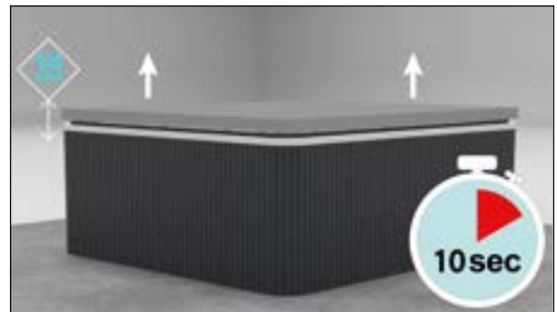
FIGURE 61: RAISE COVER 1/4" TO RELEASE SEAL FROM CLIPS
