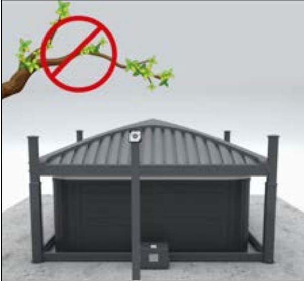
FIGURE 42: RAISE 8" — MAKE SURE COVER LIFTS EVENLY
