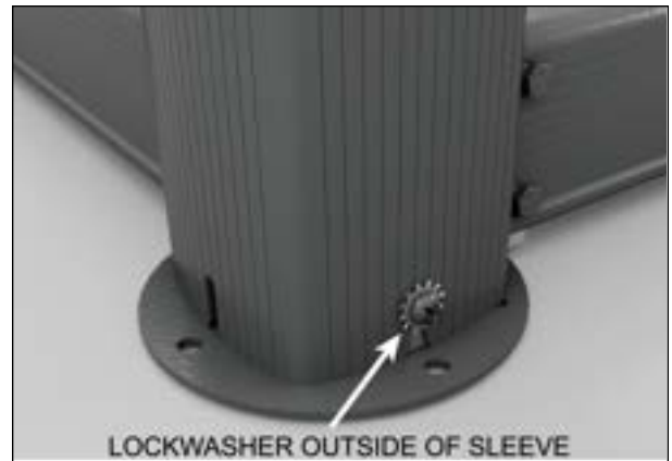
FIGURE 90: LOWER SLEEVE AND TIGHTEN SCREW
