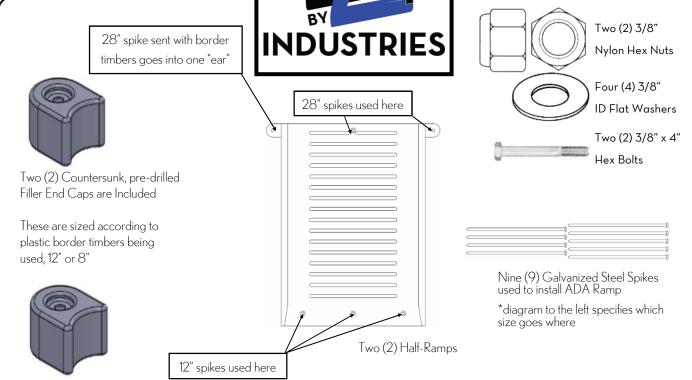
This ADA Full Ramp has been designed to work universally with any manufacturer's plastic border timber, provided its method of attachment involves a 3/4" diameter steel spike. You have the freedom to use 6", 8", or 12" plastic playground border timbers because the attachment point sits BENEATH the timber.
