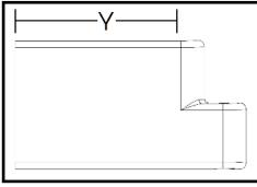
Measure from the OPEN end of the adjustable end cap, NOT the spike location to achieve measurements provided in the chart.
