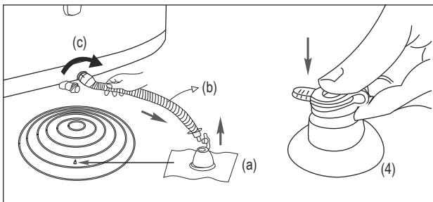
1. Open the air valve (c) on the spa pool. Ensure that you select the black one. Open the air valve (a) on the bladder. Insert the inflation hose (b) into the valve.
