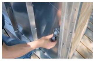
Screw the assembled pieces into the hole on the bottom of the tub.
