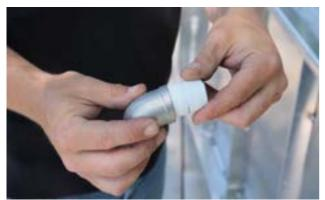
Screw the short pipe into the elbow.
